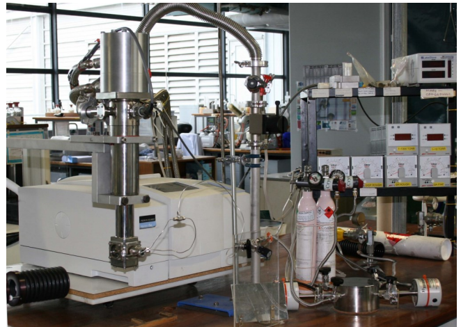
System set up for Matrix Isolation. Mixing chamber lower right. Expander and sample can be manually rotated with respect to the shroud and window. Clamped shroud stays stationary during sample rotation.
