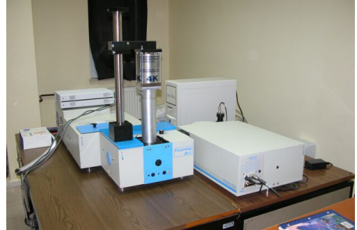
Displex installed on a spectrometer.
