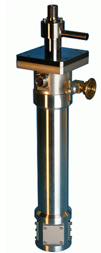
The above picture shows a cryocooler with a vacuum shroud, radiation shield, and sample holder installed.
